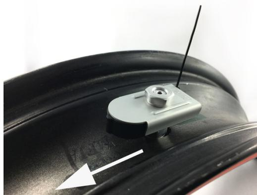
The I2M TPMS sensor is supplied with the code TPS8 for the version with 8.5mm diameter adapter valves and TPS11 for the version with 11.5mm diameter valves adapter. In both cases the valve is **NOT** included. The sensor is the same in the two models while the adapter varies, which can still be purchased separately (AD8 and AD11 respectively for 8.5mm and 11.5mm valves). The sensor is supplied with the aluminum protection to be mounted as shown in the figure.
